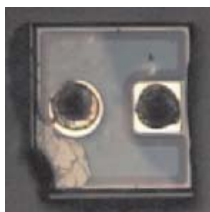
Sample surface after depackaging Die size: 300 x 300µm
