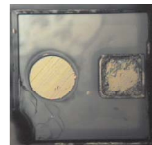
Sample surface after polishing
